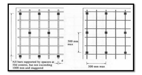
WHEEL SPACING IN COLUMN CONSTRUCTION (d = bar diameter)
